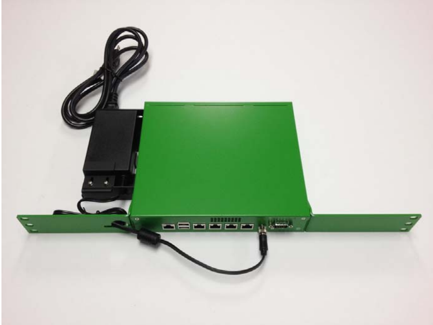
Figure 3 Assembled AG 2400 rack mount kit ports faced forward
