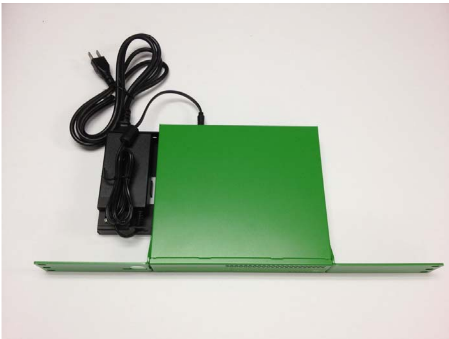
Figure 4 Assembled AG 2400 rack mount kit bezel faced forward
